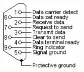
Figure 1: RS232 DB-9 pin outs
