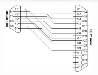
Figure 3: RS232 DB9 to DB25 converter
